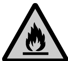
Caution, risk of fire, R290
